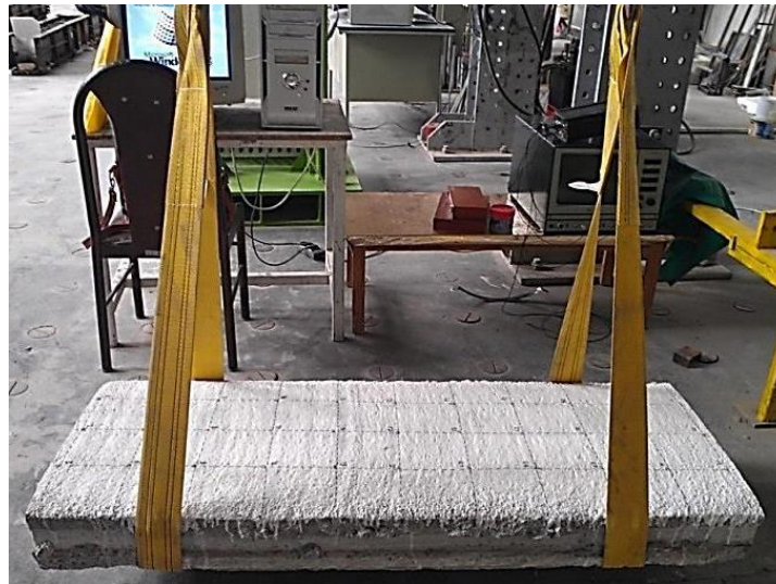
Fig. 5. Conducting modal testing on prestressed concrete slab specimen in a hanged position [51].
