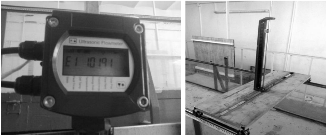
Fig. 1. Ultrasonic Flowmeter and Point Gage.
