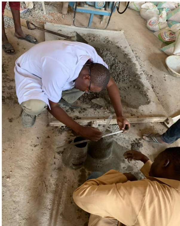
Fig. 6. Measurement of concrete slump.
