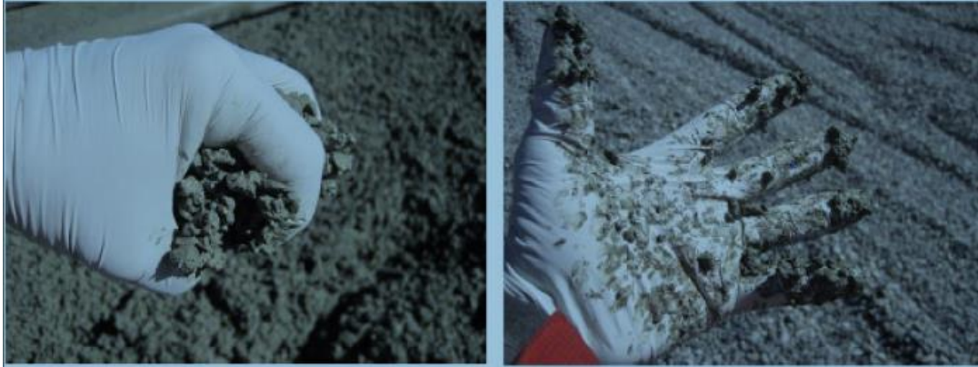
Fig. 2. Hand Squeeze pervious concrete workability evaluation [24].
