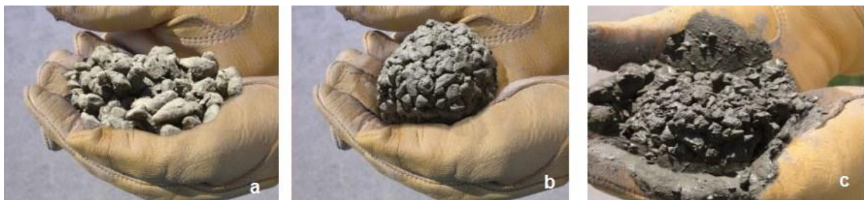
Fig. 1. Visual Inspection Approach for workability [1].
