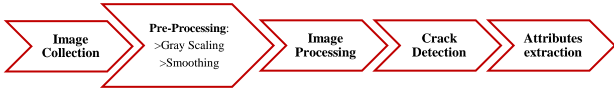
Fig. 3. General structure of crack detection through image processing proposed by Mohan and Poobal [9].
