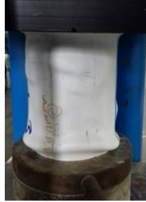
Fig. 1. Deformation of CFPT under load.
