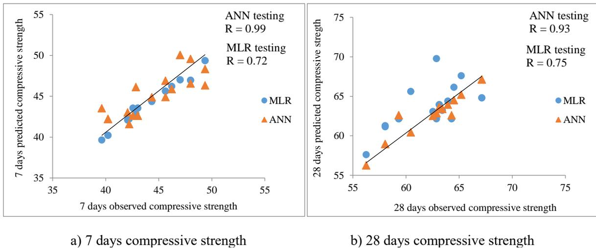
Fig. 7. (a-b) Comparison of predicted vs observed values of M50 concrete grade in testing
