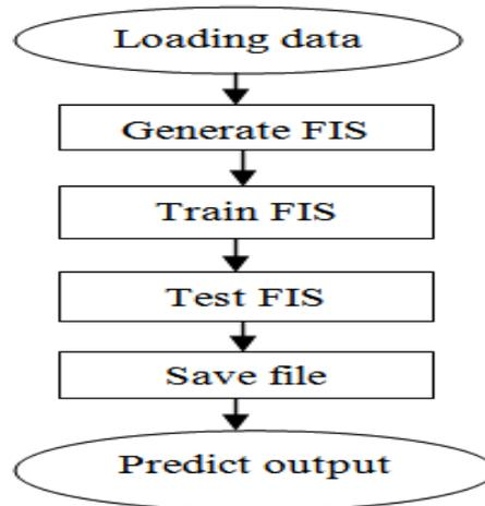
**Fig. 4.** Flowchart for development of ANFIS model
