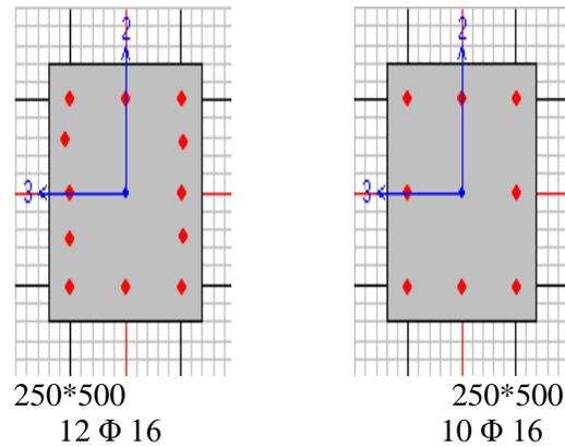
Figure 12: Design of some columns before adding seismic Loads
