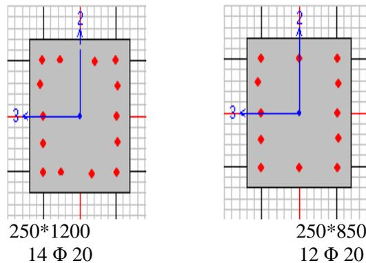
Figure 14: Design of some columns after adding seismic loads
